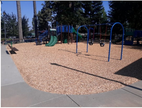
Figure 6. TARC playground with added fall material.
