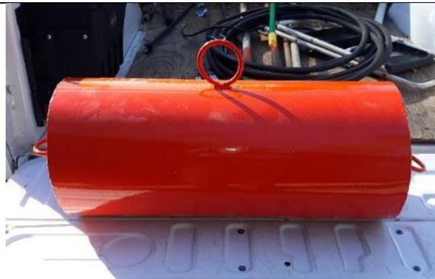
Figure 14. Refurbished pipe buoy.
